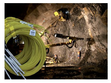
NONEL LP is a non-electric blast-initiation system series with long intervals, especially intended for drift and tunnel blasting. At this kind of blasting operations it is of great importance that delay time between intervals is sufficient to give the rock enough time to move forward without stopping.
